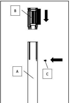
1. Press belt cartridge into pole by lining up channels with topper.
